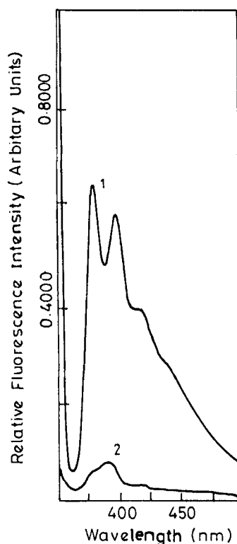
Figure-1. Fluorescence spectra (1) oligonucleotide-pyrenyl conjugate; (2) N-(3-Pyrenyl)maleimide at a concentration of 3 nmole/ml.
